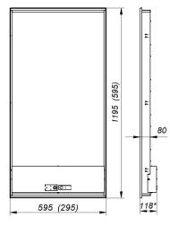
The luminaire's height 118\* is for the version with an emergency module.
